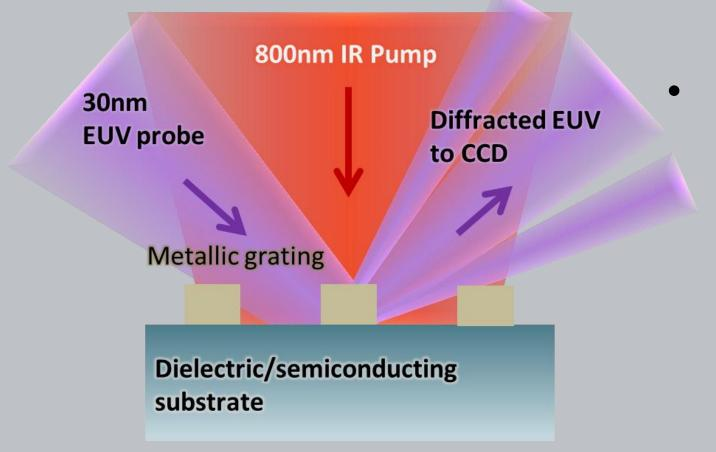
Discovered completely unanticipated regime of nanoscale thermal transport where small heat sources can dissipate heat more quickly if spaced close together rather than far apart
